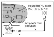
Before connecting or disconnecting the cord, stop the tape and switch [SELECTOR] to "TAPE/ OFF" to turn the power off. The memory batteries are worn out faster if the cord is disconnected with the power still on.
